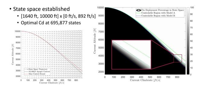
Previous ADS design established state space for Cd and ability to control apogee with respect to:
