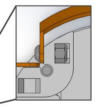
**Bolt and Lock Nut** A lock nut is epoxied to the columns where a bolt can secure the flap to the assembly, acting as a hinge.
