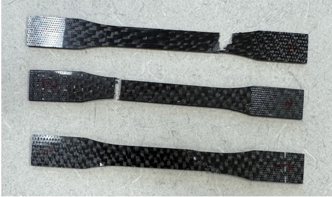
Fig. 8 Carbon fiber epoxy specimens: 1, 2, and 3 after tensile testing.
